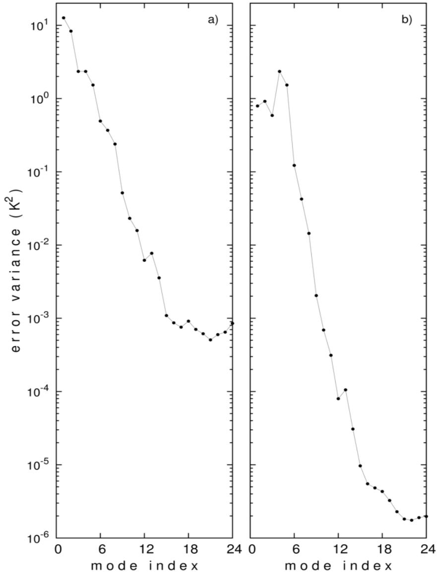
Left-hand panel: spectrum of  $HPH^T$  if the bkgd-error is defined using analytical modes all having the same amplitude.
